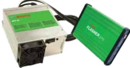
The Flasher Pro Vehicle Interface Module (VIM), along with OEM programming application software, provides dealer-level programming capabilities for all makes, all models at a fraction of the cost of a proprietary OEM dealer diagnostic tool.
